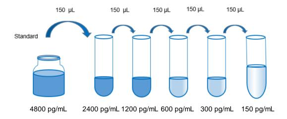
**Note**: If samples generate values higher than the highest standard, please dilute the samples with Sample Diluent and repeat the assay.
